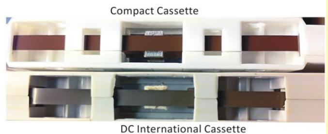
**Figure 2.** CC and DCI tape recesses compared.
