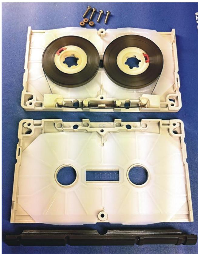
**Figure 1.** DCI cassette disassembled.
